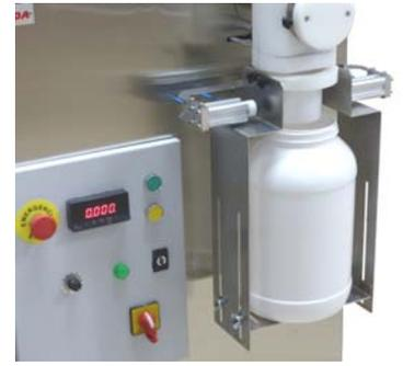
*Machine specially indicated for the dosage and weighing of powdered products, such as flour, bread crumbs or similar.*
